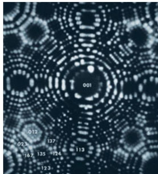
Courtesy of David Seidman. 1973 platinum micrograph, each dot is the image of an individual platinum atom.
